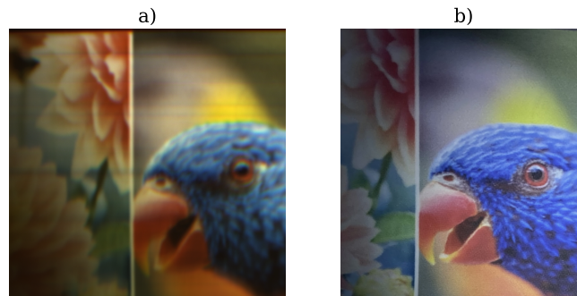
Figure 2.3: a) Reconstructed RGB image from object (colorful parrot) with a hyperspectral camera, b) A photo made with a phone.
